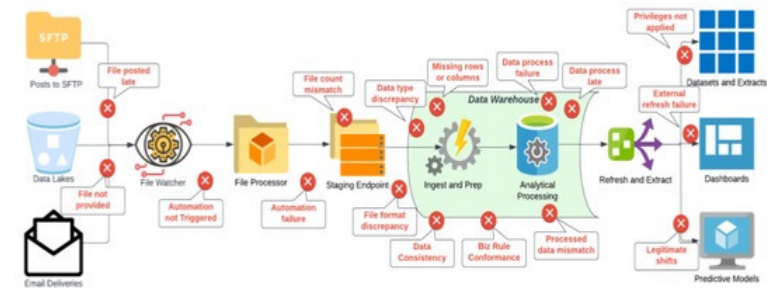
Figure 8: Problems can occur anywhere in the Journey data takes form source to value. Testing in key.
